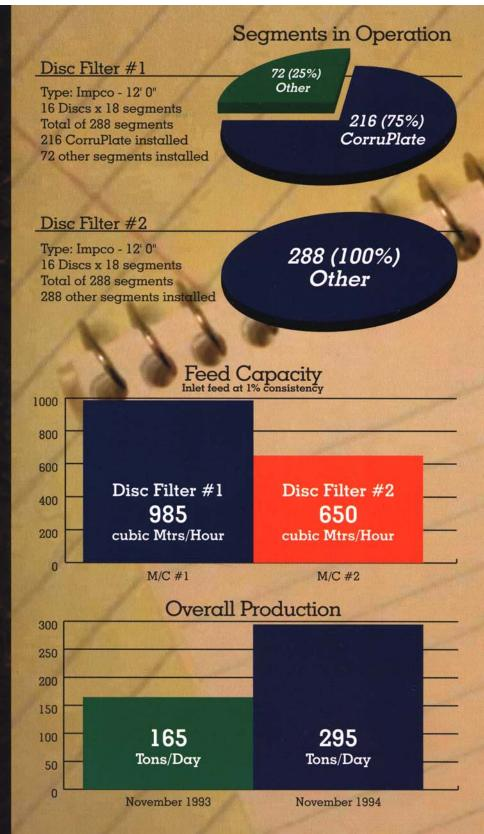
The above results were obtained from a recycling / de-inking mill that started replacing their old segments with CorruPlate in May 1994. Completion of #1 filter is expected in February 1995.
